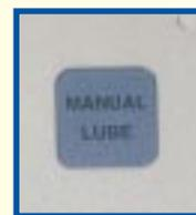
*Manual lube button initiates a lubrication cycle which allows easy testing and servicing of the system.*
